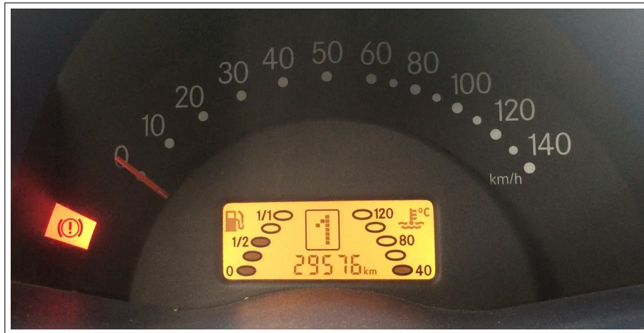
Figure 4.4: Attack on the transmission display. The engine was not running but the indicator showed gear 1. The control lights were switched off and the fuel level was increased.
