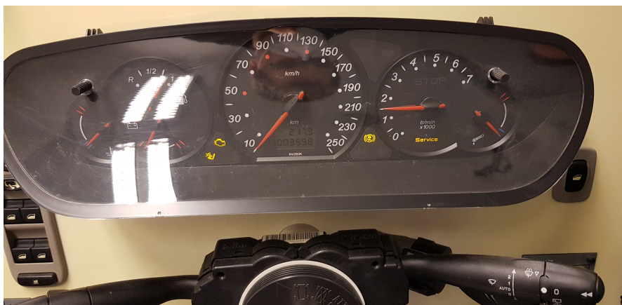
Figure 2.8: The attack of the tachometer displays different rpm than the real one.
