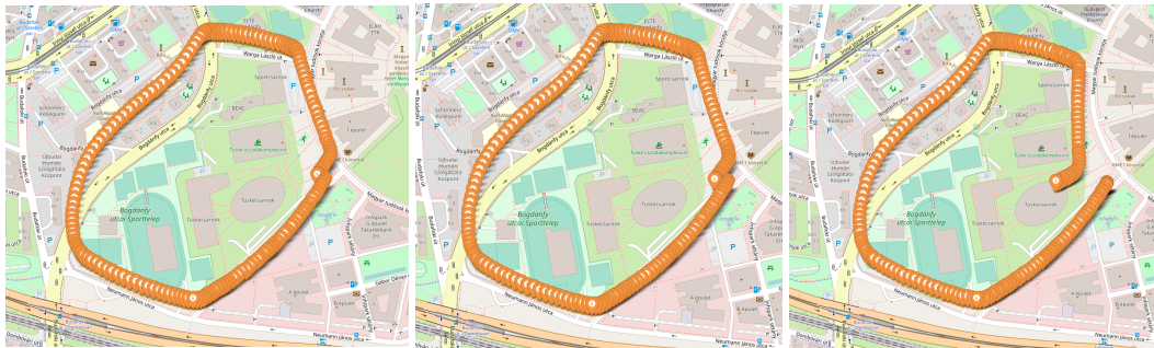
(a) Smoothing window: 0.201s (b) Smoothing window: 1.608s (c) Smoothing window: 6.4s
