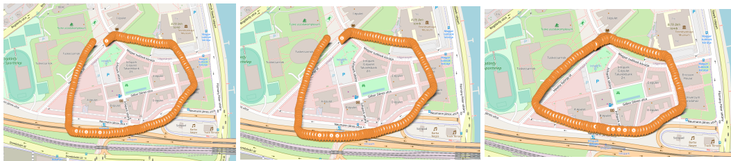
(a) Smoothing window: 0.201s (b) Smoothing window: 1.608s (c) Smoothing window: 6.4s
