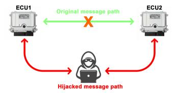
Figure 2. The concept of a MITM attack in the automotive industry.
