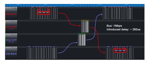
Figure 7. Simultaneous message transmission in both direction.
