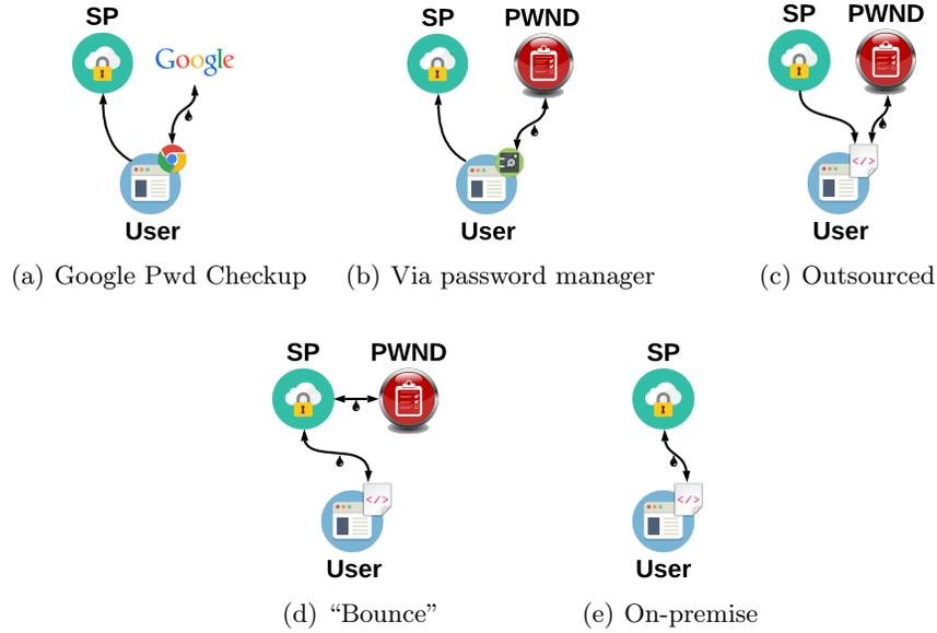
**Fig. 1.** PWND architectural alternatives: initiated either by the user or by the service provider
