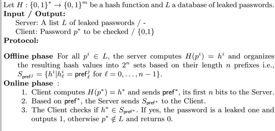
**Fig. 2.**  $K$ -anonymity preserving protocol for checking whether a password has already been leaked (for  $K = 2^{m-n}$ ).
