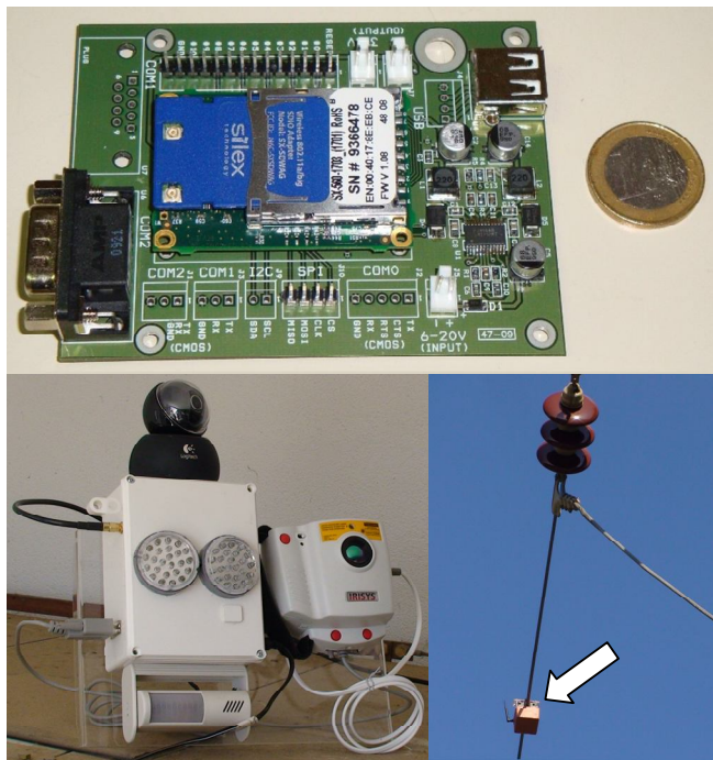
Figure 2. Top: Silex sensor with PCB; Bottom-left: Sensor with webcam, infrared camera, LED light and movement sensor; Bottom-right: Sensor hanging on a 15 KV line, harvesting energy from the line.
